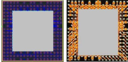
Figure 2. PKG drawing and micrograph of test vehicle of 9x9mm eWLB.
