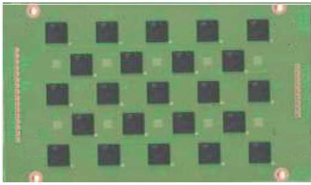
Figure 4. Board level reliability test board with surface mounted eWLB packages.
