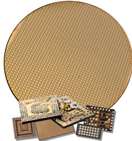
Figure 1. 300mm eWLB carrier and various units.
