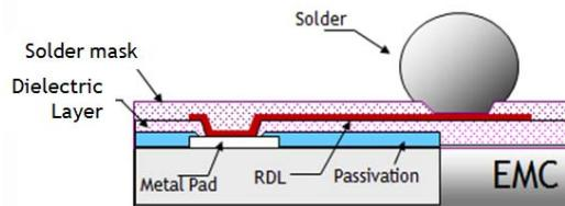
Figure 3. Schematics of eWLB package.
