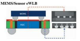
Figure 7. 3D eWLB for MEMS/Sensor Devices [2]
