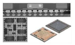
**Figure 5.** 3D SiP eWLB-PoP with Discretes in Interposer on Top Package
