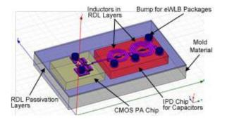
**Figure 10.** Illustration of a PA Die and Silicon IPD Die Embedded in Mold Substrate
