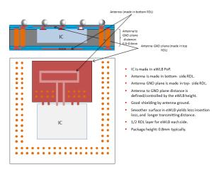
Figure 8. Double Sided RDL eWLB AiP Module
